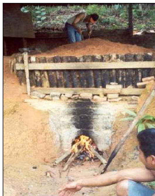
Phot 5. Permanent kiln which made by brick (design by Yoshimura)
