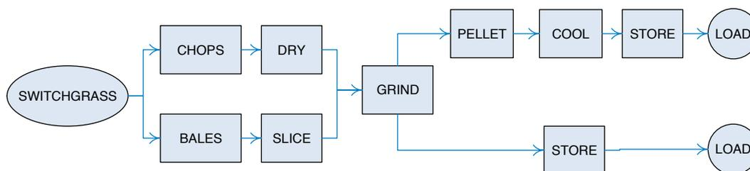
Figure 2. Flow diagram for densification of biomass to pellets or to small particles.
