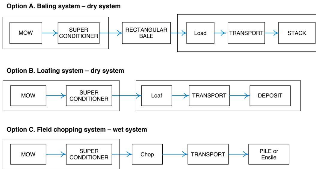
Figure 1. Advanced options for harvest and collection of switchgrass. The outer box (thin line) indicates that these operations can be assembled in a single piece of equipment.
