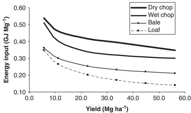
Figure 7. The unit energy input for four harvest scenarios as a function of yield (crop density).
