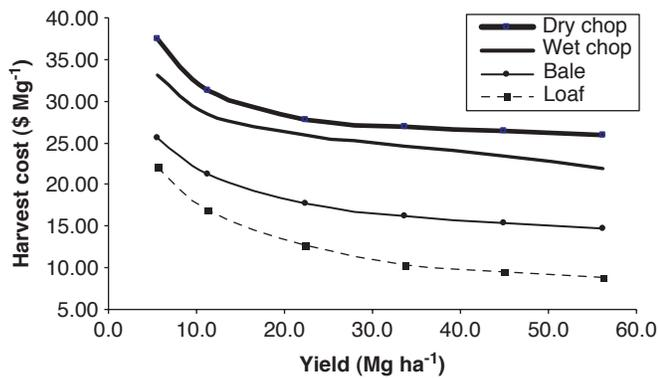
Figure 6. The unit cost of four harvest scenarios as a function of yield (crop density).
