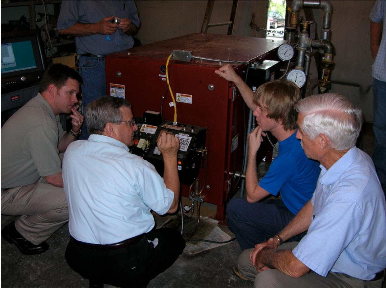
University of Georgia Engineers work with Engineers from Clean Burn and Underwriter's Laboratories to optimize an instrumented Clean Burn used oil burning boiler to efficiently burn freshly rendered poultry fat.
