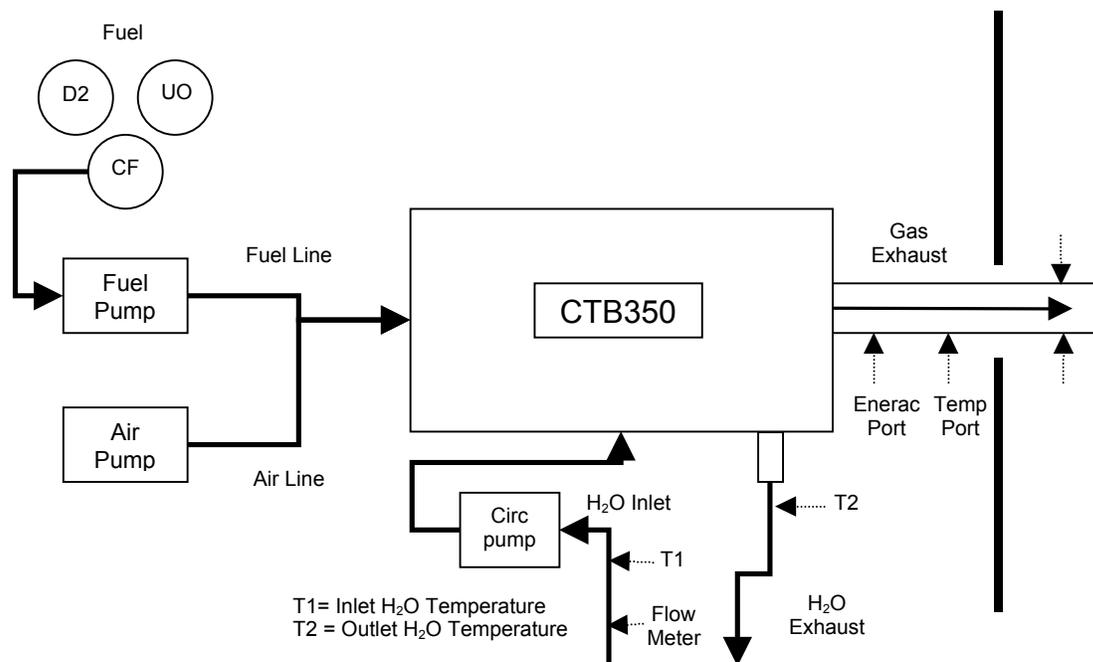
**Figure 1.** Bloc diagram of CB 350CTB Coil Tube Boiler, fueling system and hydronic system.
